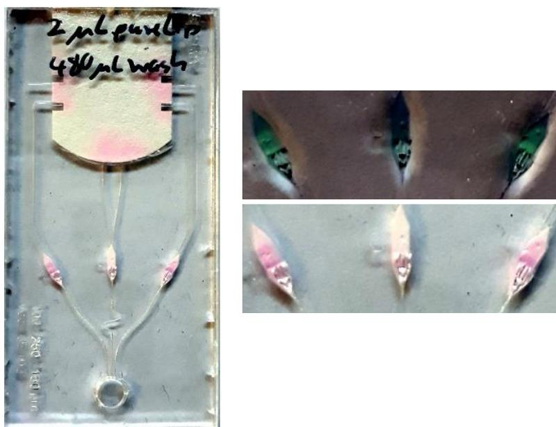
Figure 3: Left: Microfluidic chip with polystreptavidin-modified nitrocellulose membranes (left and right) and unmodified NC membranes (middle) after addition of 2  $\mu\text{L}$  8.87 mM biotinylated liposomes and washing with 480  $\mu\text{L}$  liposome complement buffer. Right: Zoom-in to the NC membranes (upper picture: colors inverted).
