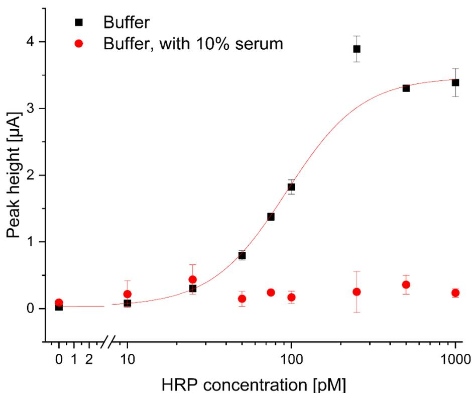
Figure 5: Different concentrations of HRP with 15  $\mu\text{M}$  TMB in LCB with and without 10% human serum (pooled); Peak heights at 0.30 V determined via SWV (square-wave voltammetry). Measurements performed in triplicates.
