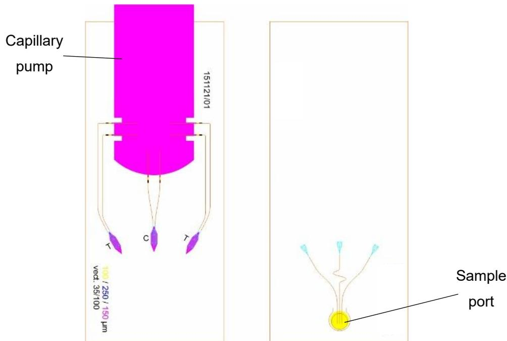
Figure 1: Designs for a multiplexed microfluidic system, laser-engraved into PMMA plates. Left: Top plate; right: bottom plate. Magenta marks the integration of the capillary pump, at violet, (T) polystreptavidin-modified (left and right) or (C) unmodified (middle) nitrocellulose membranes are integrated.
